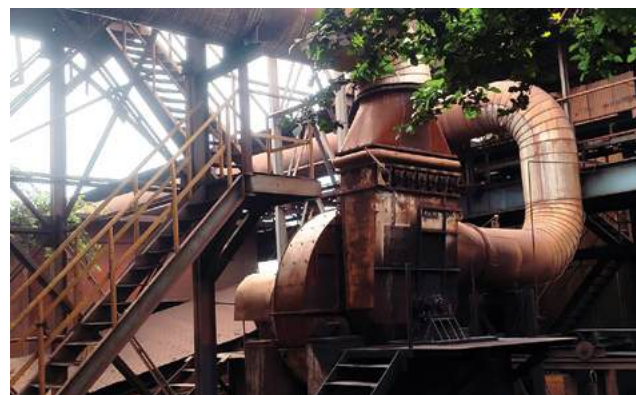
Coke Drying System to enhance coke calorific efficiency and reduce moisture-related issues
