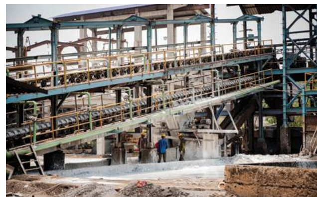
Double-Strand Pig Casting Machine to improve casting throughput, reduce manual intervention and improve product uniformity
